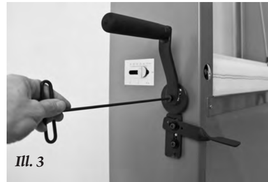
III. 3 See the quick stop lever installed on the left side of the machine. The configuration is slightly different from the right hand side.
