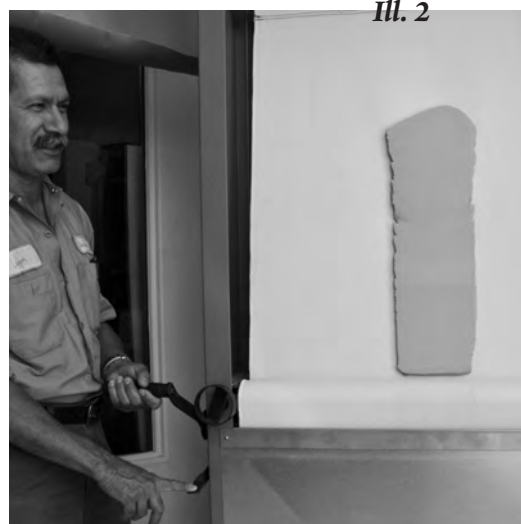
III. 3 See the quick stop lever installed on the left side of the machine. The configuration is slightly different from the right hand side.
